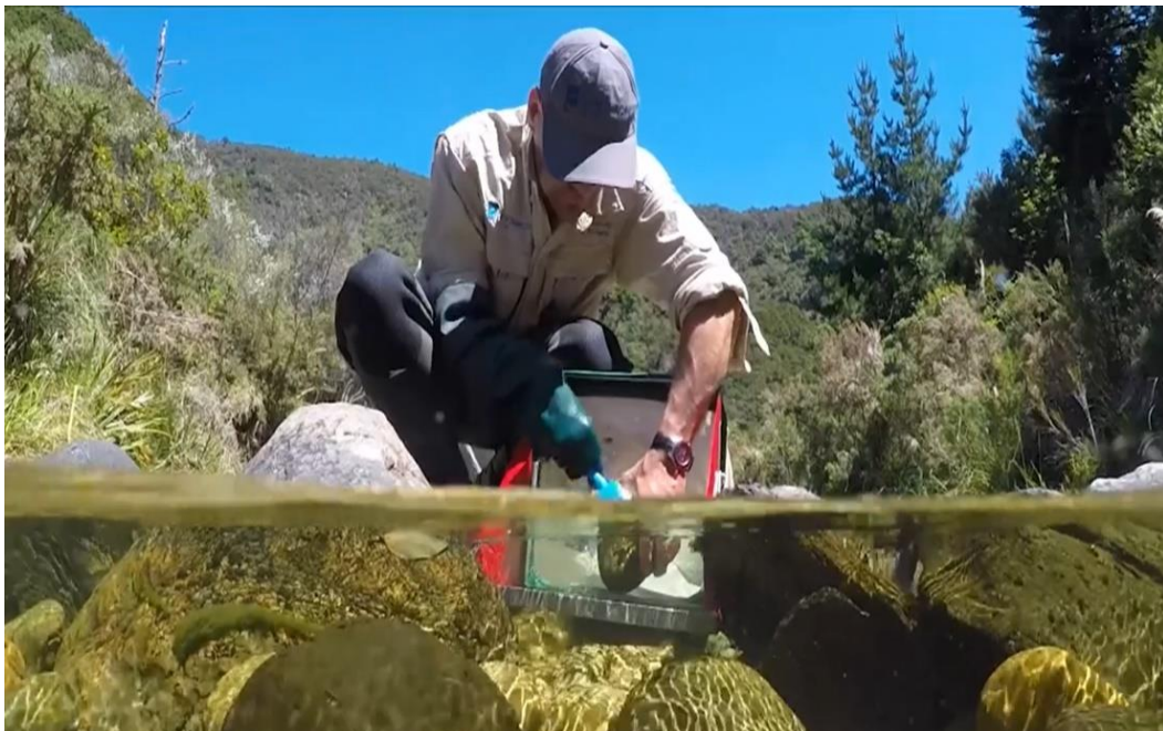
Figure 2. A macroinvertebrate sample being taken using a Surber (box) sampler. Note the use of scrubbing brush to dislodge animals from stone surfaces.
