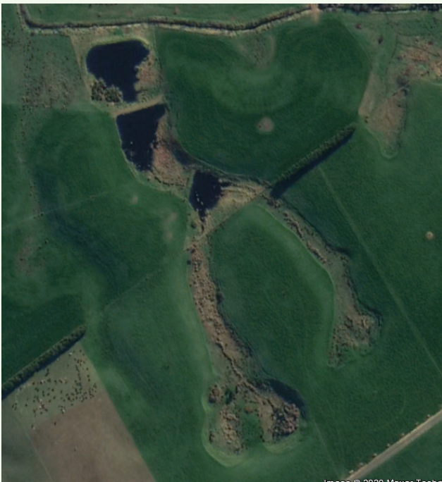
IMAGE 2: This image is the same as location as the previous image approximately 4 years after the completion of the sediment trap structures. You can easily see the pond areas where water velocity is slowed to allow suspended sediments to drop.
