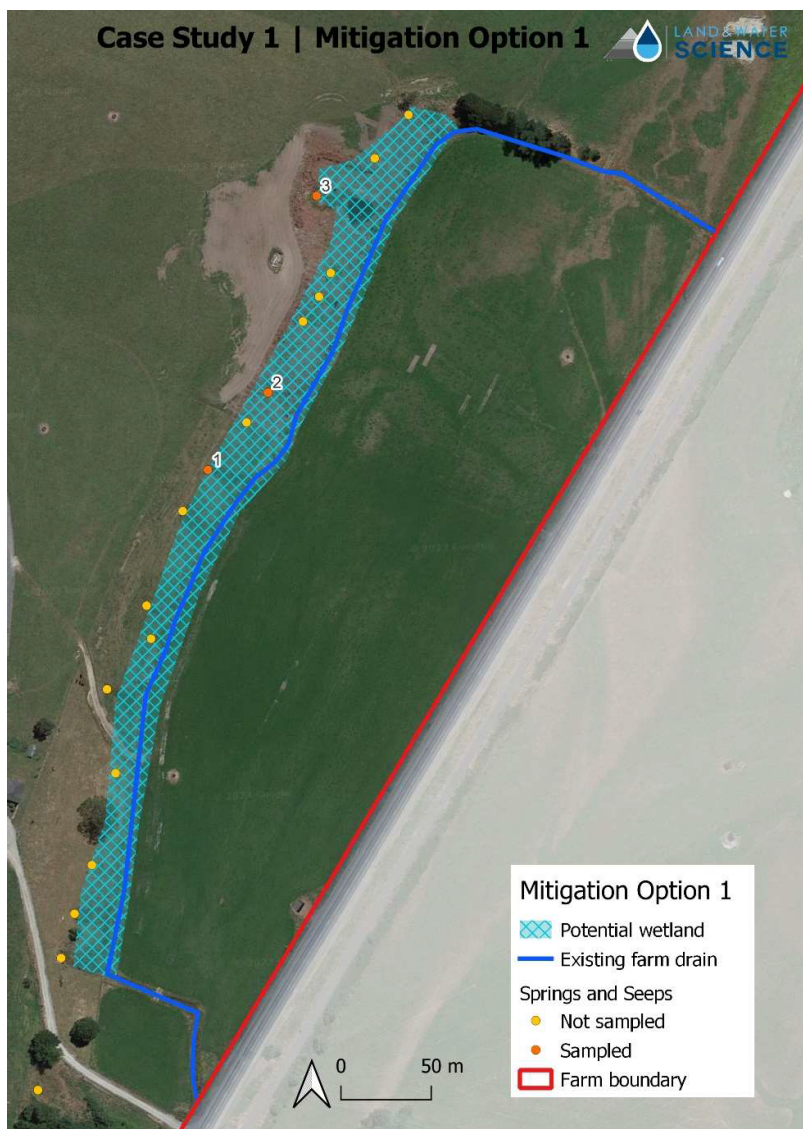
Figure 18. Potential wetland area (1.5 ha) on the sidling. Modification to the existing farm drain would be required to develop the seepage wetland system. The springs sampled are identified with sample numbers.
