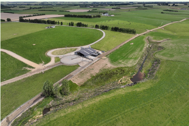
IMAGE 1: Looking upstream towards the west. You can see the swale, critical source area or natural low point in the landscape above the construction area where overland flow will collect before flowing through the sediment trap system.
