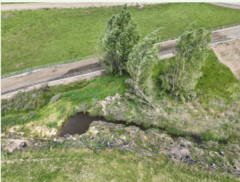
IMAGE 4: A close up of the second, smaller sediment trap in this series. Water from the outlet flows into an open drainage channel and into an adjacent waterway.
