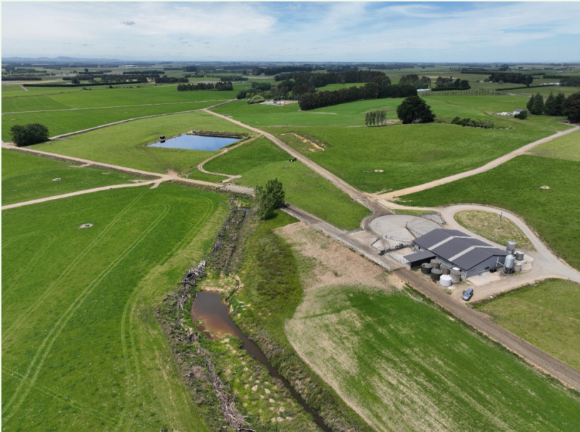
IMAGE 2: Looking downstream towards the east. You can see the larger containment area at the top of the series in the center of the image. The overflow channel located to the site of the sediment trap flows down to a second smaller sediment trap.
