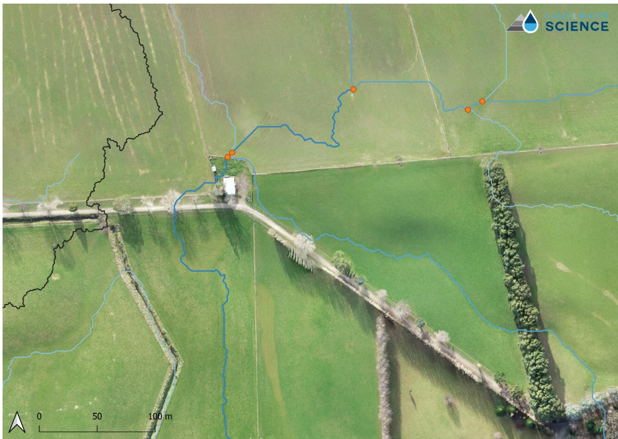
Figure 9. Roslyn Downs – zoomed in view of several priority nodes identified. Junction nodes (orange circles) identify where drainage channels converge or join.
