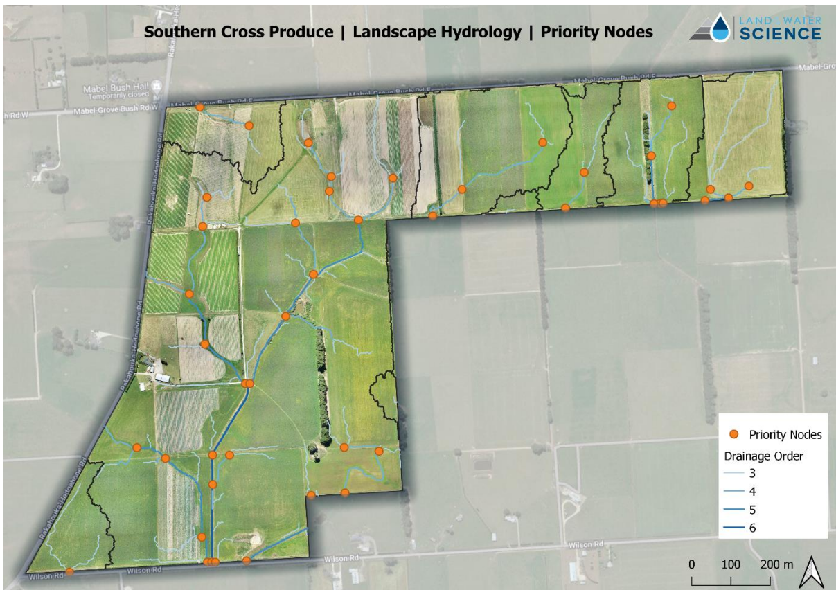
Figure 8. Southern Cross Produce - landscape hydrology – drainage orders 3 - 6 only (i.e., the major drainage channels within the farm property), plus the related junctions and discharge nodes.
