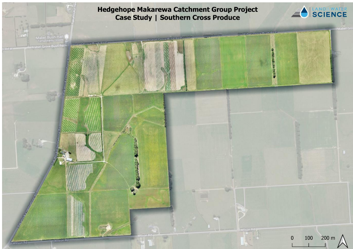
Figure 3. Southern Cross Produce. The photogrammetry survey generates an orthomosaic output at 3cm resolution, producing a Digital Elevation Model of 12cm/pixel, with a vertical geolocation accuracy of 0.02cm.
