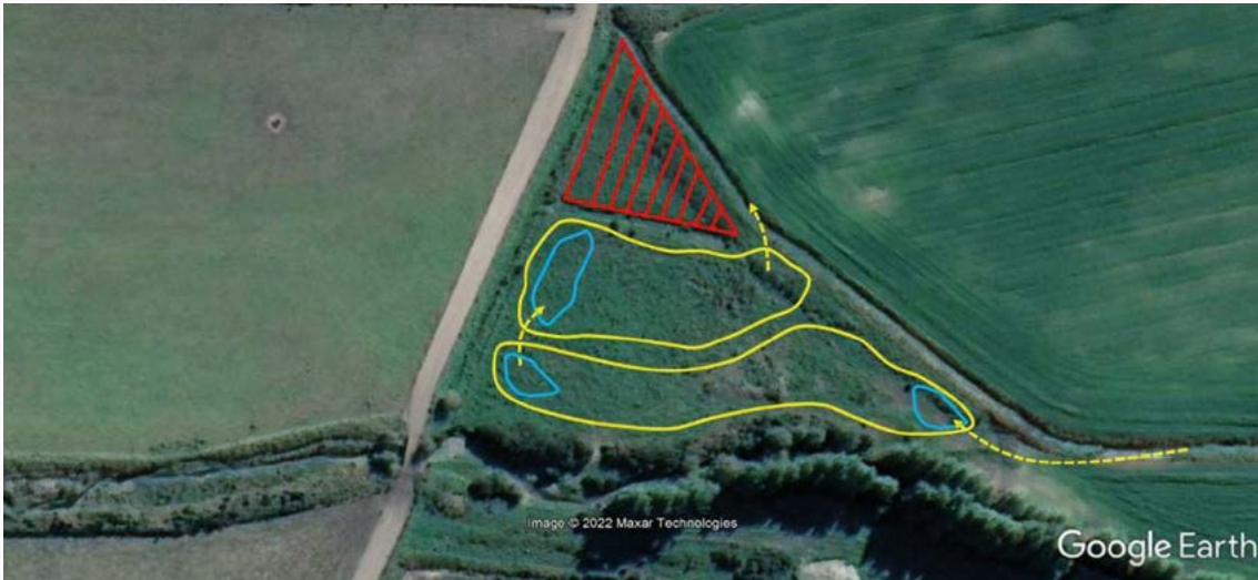
Figure 1 - The proposed wetland areas. The proposed wetland is divided into two cells outlined in yellow. Inflow, outflow and inter-cell connections are shown as dashed yellow arrows. Zones outlined in blue are deeper areas (1-1.5 m) for improved flow distribution and capture of any residual solids. The red hatched triangle is an area identified by the farmer as not available for wetland construction.
