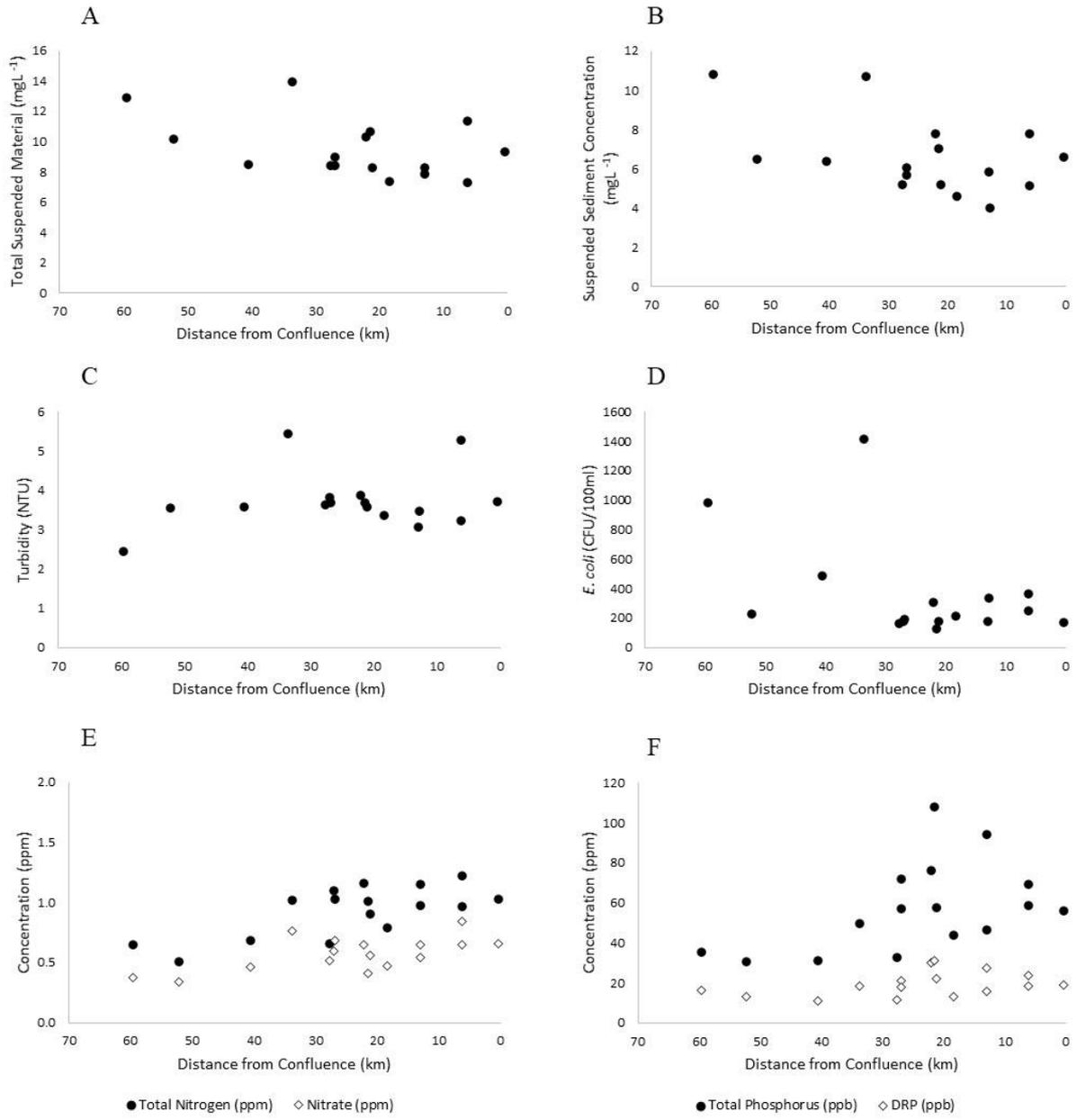
Figure 0.1 Shows the distance spread of the concentrations of measured water quality variables A) total suspended material B) suspended sediment concentration C) turbidity D) *E. coli* E) total nitrogen and nitrate F) total phosphorus and dissolved reactive phosphorus.
